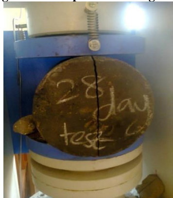
Figure 4.2 compressive strength test
